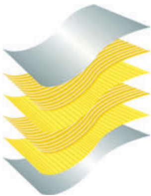
4 fiber and resin plies consolidated with thermo-plastic film to protect the composite package
